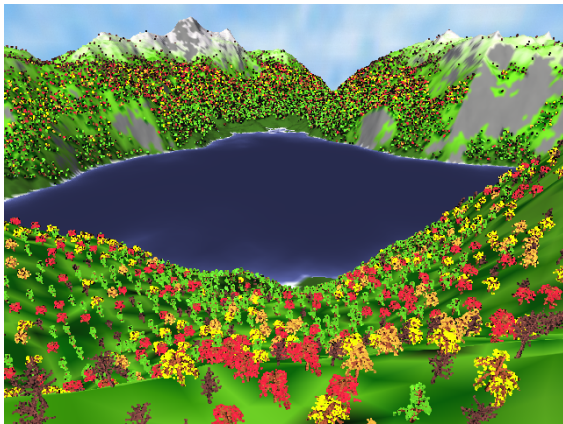
(c) Landscape scene ( 4.1 \times 10^8 triangles), splatting, d=2 , diffuse illumination model, rendering time: 262 msec
